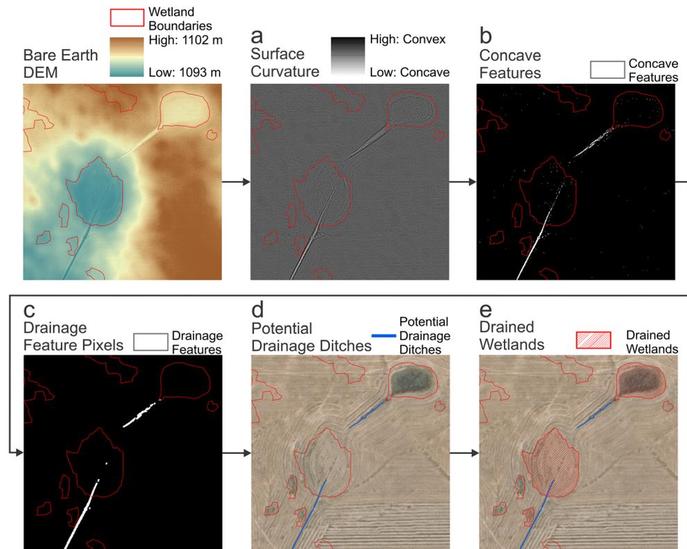
break point, consistently appearing when data were binned into four or more classes. The data were reclassified to a binary map with smoothed curvature values less than or equal to  $-6.61$  (representing potential drainage ditches) reclassified as “1” and all other values (representing other surfaces) reclassified to “0”.
